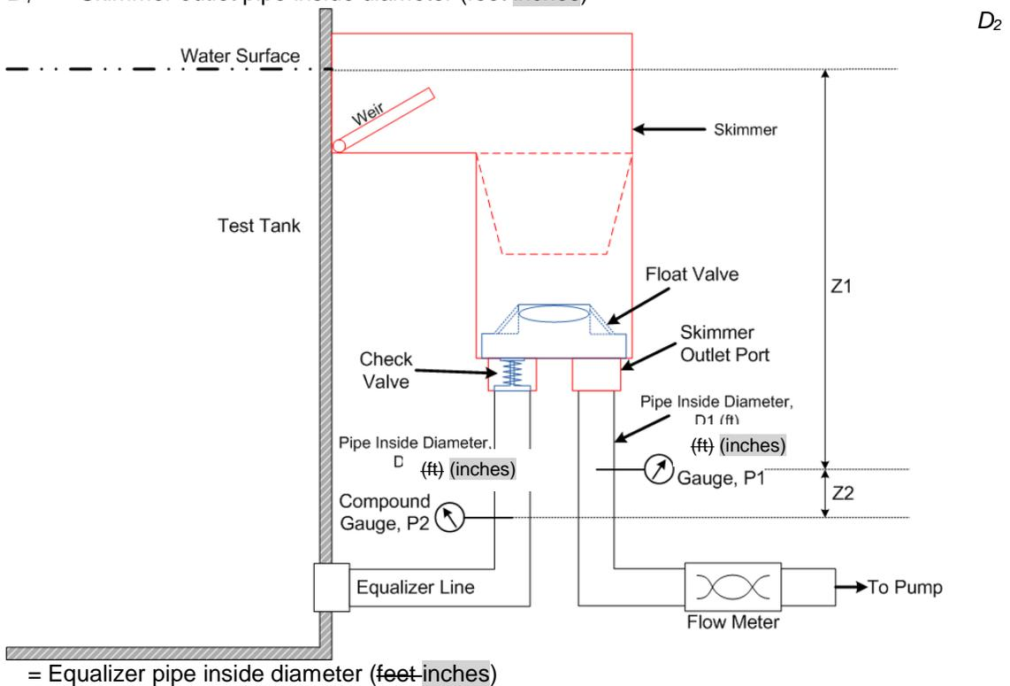
**Figure 10 – Skimmer head loss & equalizer performance test setup (normal operation)**
